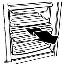
Pull out to the stop, lift the front, and pull again.
